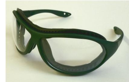
On February 06, 2019, COLTS Laboratories received Spectacles: LIBUS FALL DUAL from LIBUS PPE. From February 11, 2019 through February 21, 2019 COLTS Laboratories tested these Spectacles in accordance with ANSI Z87.1-2015 to the following test protocol: ANSI Z87.1-2015 High Impact Spectacles - Base Model.
